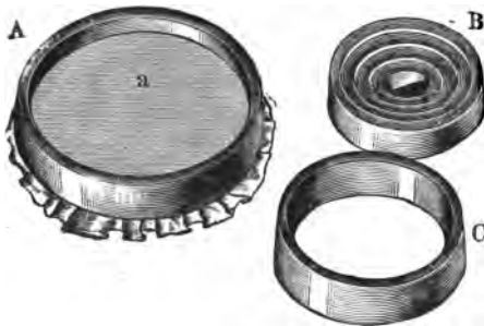
FIG. 44.—A: Vulcanite rings used for stretching a membrane which is to be silvered; B: Conical rings, the one inside the other; C: A single ring.
